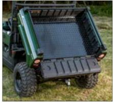
CARGO BED AND TOWING CAPACITY The PRO-MX offers a 317 kg (700 lbs) cargo bed capacity, and a 680 kg (1,500 lbs) towing capacity
